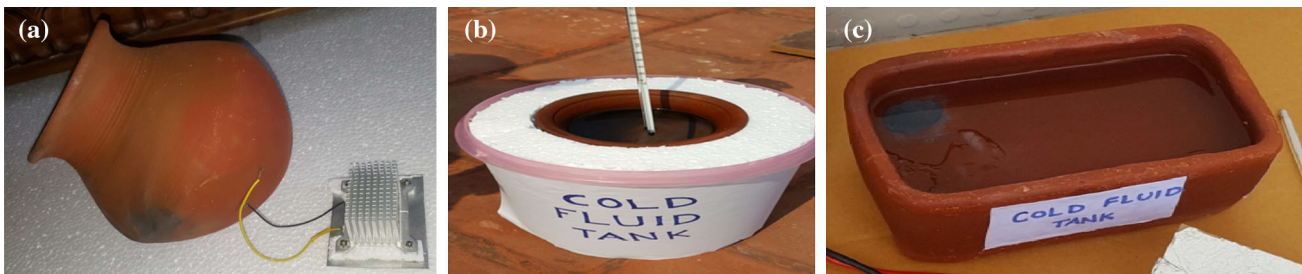
Fig. 9. (a) An earthen pot arrangement and a heat sink (b) earthen pot was placed inside a plastic container filled with thermocol alongside the wall (c) flat base rectangular shaped earthen pot.
