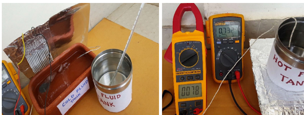
Fig. 12. Modified cold junction arrangement of TEG.
