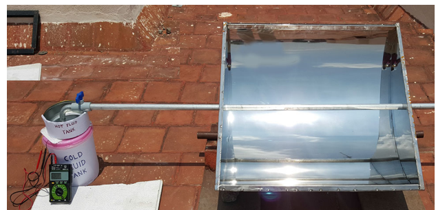
Fig. 10. Integrated experimental setup for the energy harvesting system.
