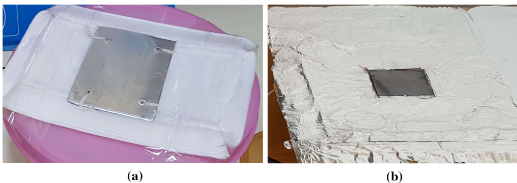
Fig. 8. (a) Aluminium plate covering the TEG (b) cardboard sheet wrapped with Al foil.
