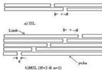
Fig.1. Investigated types of overlap arrangement a) SSL b) MSL
