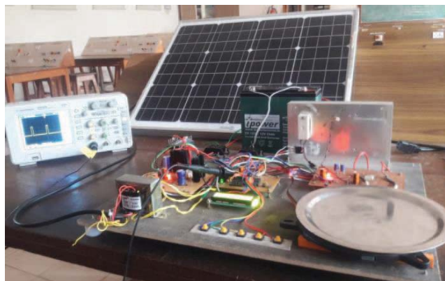
Fig 5.4 Solar Powered Induction Cooking System
