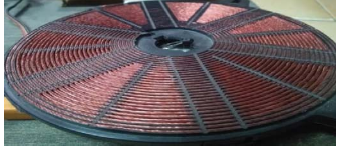
Figure 4.7 Induction Coil of 15cm in diameter with the temperature sensor
